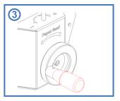
Turn the paper enter handle counterclockwise to make the honeycomb paper pass through the device.
