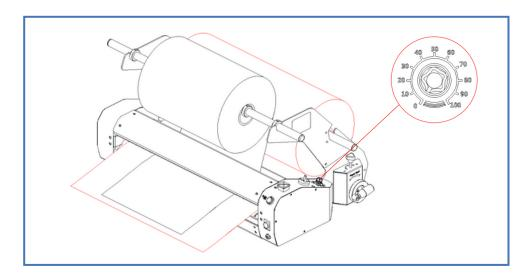
When the honeycomb paper does not stretch out shape of honeycomb holes, the adjustment handles on both sides can be adjusted at the same time to increase the resistance and adjust to a suitable state.
